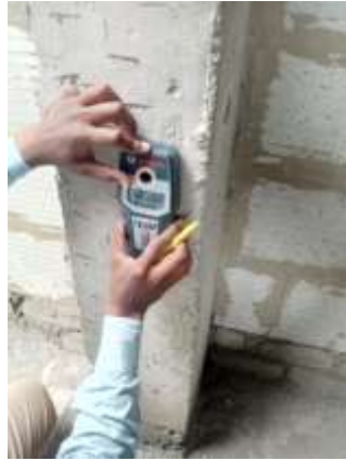
Fig I Excess Cover observed in Column
